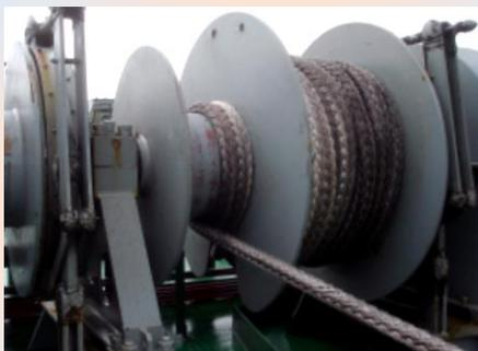
Correctly set up with at least 4 or 5 turns on tension drum
