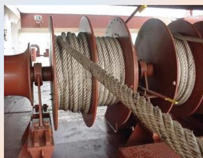
Incorrectly set up split drum with buried mooring line
